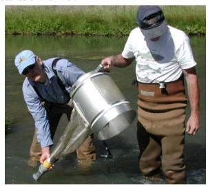
Hess Sampler with Macroinvertebrates in Container at Terminal End of Sampling Net
